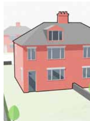
Diagram showing sensitively sized and aligned dormer
