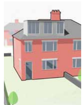
Diagram showing poorly designed oversized and unsympathetic dormer
